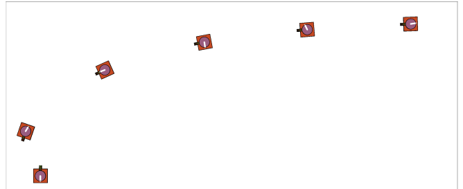
Fig. 2. Evenly timed snapshots of the Chaplygin beanie with m = a = B = C = 1 subject to the control law \dot{\alpha} = k\theta for k = 1 (top), k = 5 (middle), and k = 10 (bottom).
