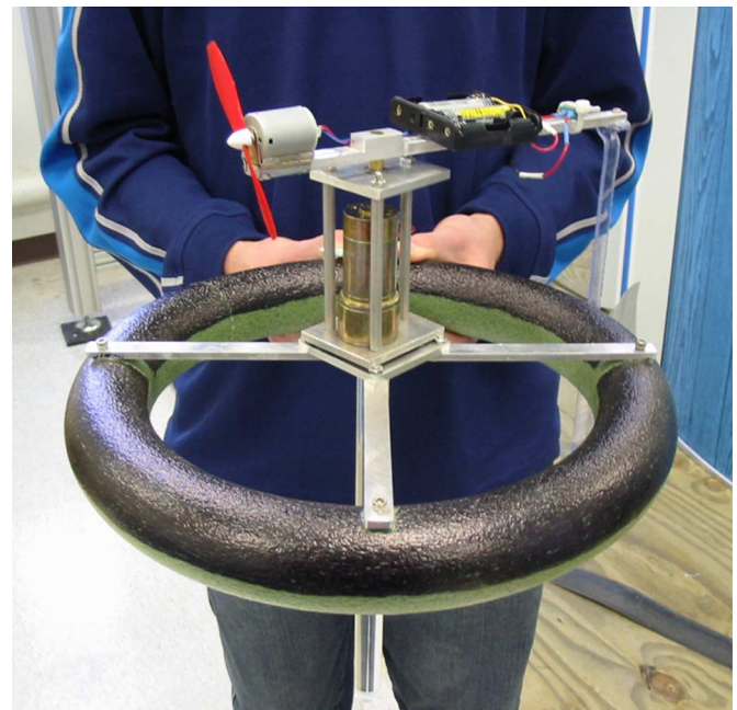
Fig. 3. Fan for passive drag cancellation.
